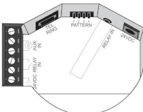
The 1128 Strobe is typically wall or ceiling mounted with concealed wiring run back to an equipment room or closet. In such cases the terminal block is used for wiring connections.
